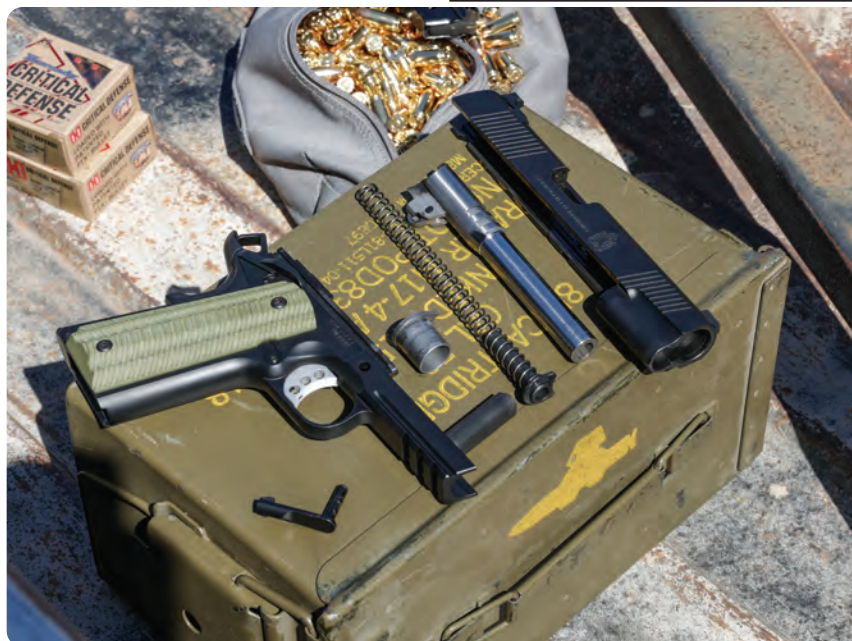
The traditional bushing system of the 1911 Operator makes fieldstripping the pistol both familiar and easy.
